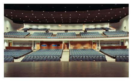
Civic Auditorium lighting once provided by 48 balcony incandescent 120 watt lamps is now provided by 14 watt LEDs. The illumination from 116 auditorium incandescent 300 watt lamps is now replaced by that from 19 watt LEDs. This saves energy costs and reduces energy consumption.
